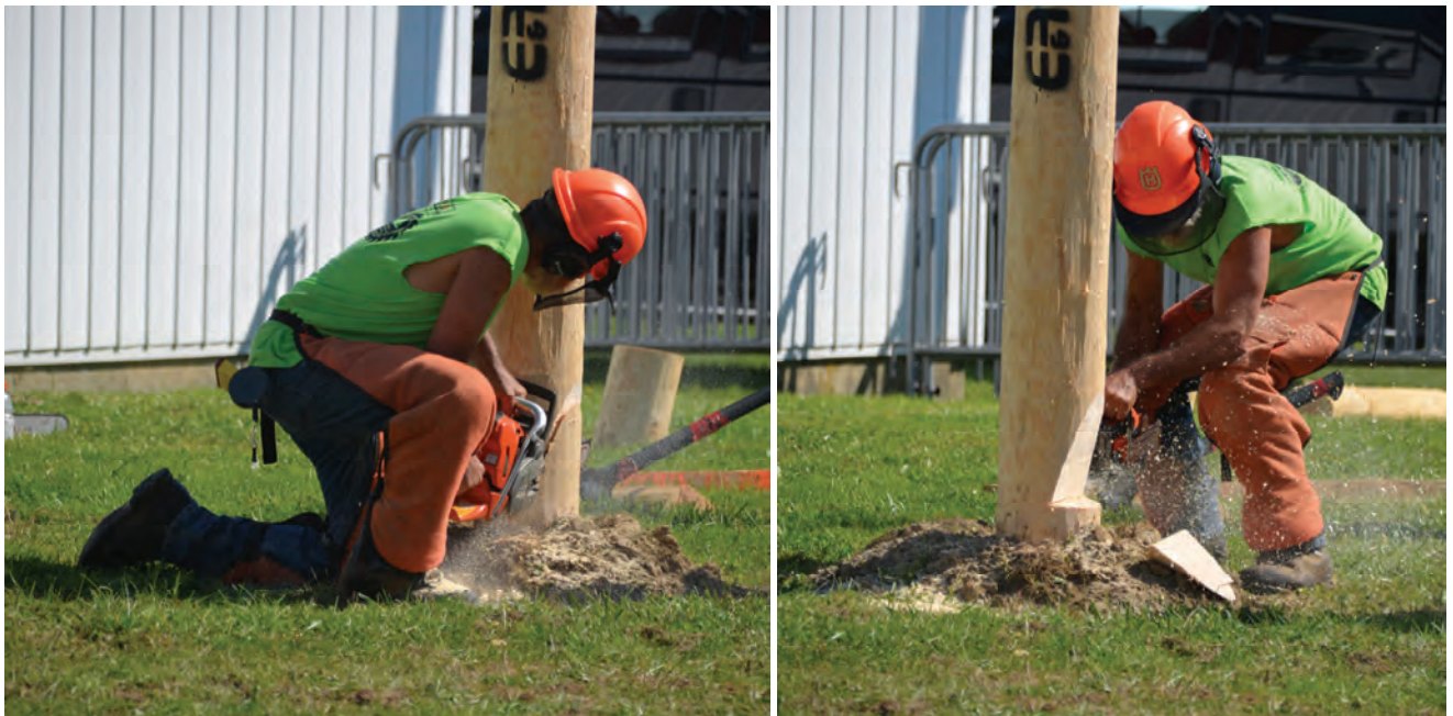
Daryl Rudgers demonstrates the safe way to drop the pole by making cuts from two sides.
