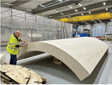
David Olivegren of Modvion inspects a modular section of the wooden turbine tower in the factory
